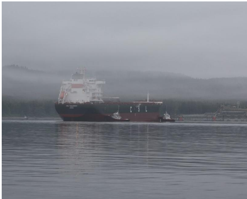
CSL Tecumseh being berthed at Port McNeill BC. Launched in 2013 from Chengxi Shipyard in Jiangyin China, she is the second trillium class Panamax-size bulk self-unloaders commissioned by the Canadian Ship Lines to haul dry goods - such as sand and gravel.
