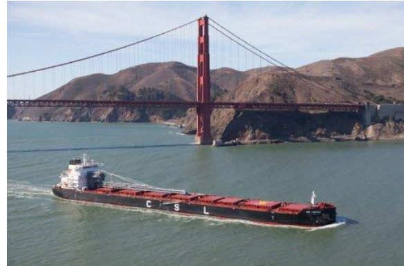
CSL Tacoma on her maiden voyage, hauling sand and gravel to Redwood City, California, Nov 6, 2013. The background view is the Golden Gate Bridge. This Canadian Shipping Line Panamax bulk carrier is similar in size and use as what would be expected to call on the pier.
